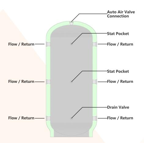
Our Buffer Vessels are designed to store heated non-potable hot water for instant demand for another system such as a radiator or undefloor heating.
